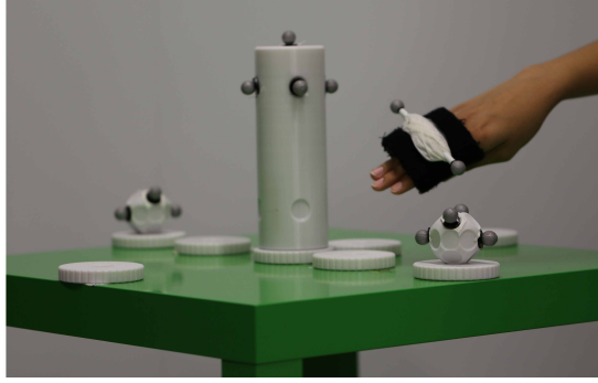
Figure 7.2: The Vicon setup showing the start, goal points, cylindrical obstacle and a human demonstrator guiding a set of markers through the environment.
